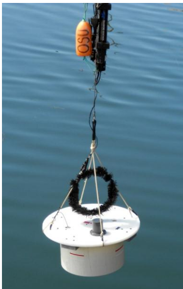
Figure 1. Image of assembled BMFC chamber prior to test in Yaquina Bay, Oregon. The cathode is directly above the chamber. Above the cathode is the acoustic modem and PMP housing with an oxygen optode sensor attached to the side, all suspended by the foam float.
