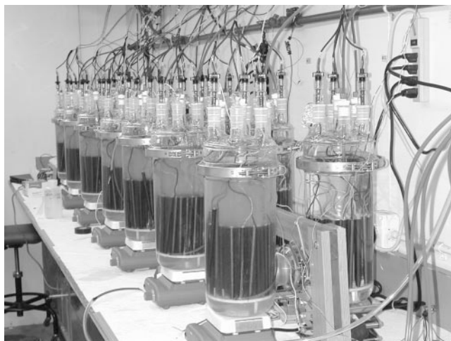
FIG. 2. Experimental setup of MFC assemblies, with anode chambers to the left on stir plates and cathode chambers to the right on laboratory jacks.
